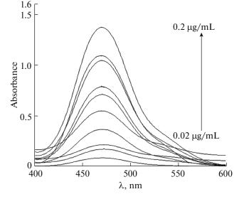
**Fig. 5.** UV-visible absorbance spectra of sediment phase in the presence of different carbamazepine concentrations.
