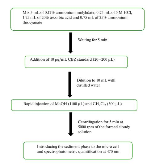
Fig. 1. Dispersive liquid-liquid microextraction procedure for carbamazepine determination.
