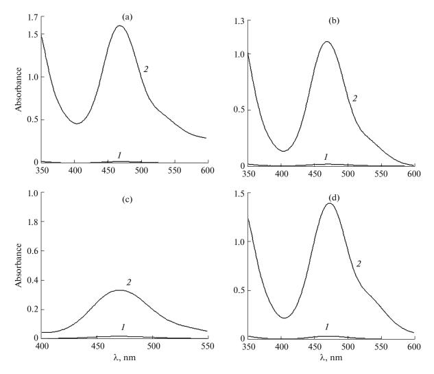
Fig. 2. Absorption spectra of extracted organic phase of  $0.1 \,\mu\text{g/mL}$  carbamazepine before (1) and after dispersive liquid-liquid microextraction (2) for standard (a), drug (b), urine (c) and serum (d).
