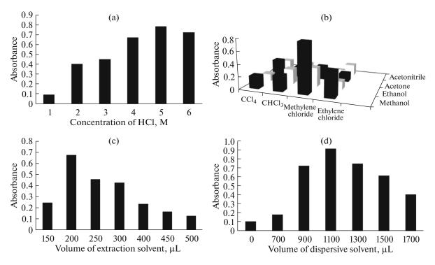
Fig. 3. Effects of hydrochloric acid concentration (a), types of extraction and dispersive solvents (b), extraction solvent volume (c) and disperser solvent volume (d).
