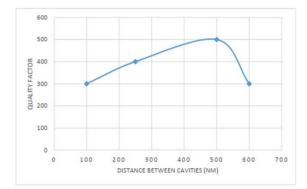
Fig. 7. Quality factor change with different distance between cavities.
