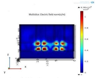
Fig. 4. Electric field distribution in the cavity.
