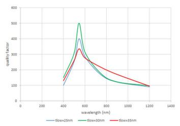
Fig. 9. Quality factor versus wavelength for different width of dielectric layer (using silver).
