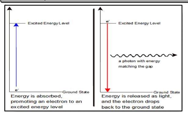
• Under constant and specific and controlled condition , the intensity of the light is proportional to the number of excited atoms which is proportional to the total number of atoms in the flame the sample concentration .
