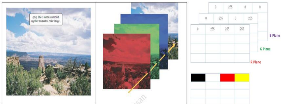
Figure (17) :A color pixel vector consists of the red, green and blue pixel values (R, G, B) at one given row/column pixel coordinate( r , c)
