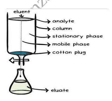
Chromatography is based on the principle where molecules in mixture applied onto the surface or into the solid, and fluid stationary phase (stable phase) is separating from each other while moving with the aid of a mobile phase.
