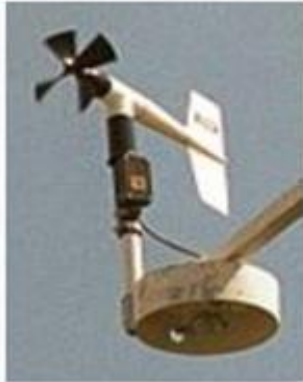
Helicoid propeller anemometer incorporating a wind vane for orientation
