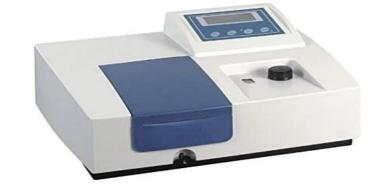
The sample should then be assessed by using spectrophotometer (an instrument that measures the absorbance of light by a colored sample at certain wavelength)
