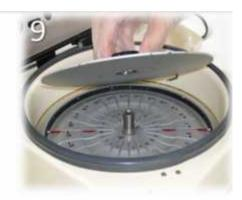
Screw the metal cover (plate) on firmly. Close and secure the centrifuge lid.
