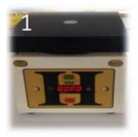
Switch on the centrifuge at the wall. Some centrifuges also have a switch on the machine. Open the lid – some centrifuges have a button while others have a catch.
