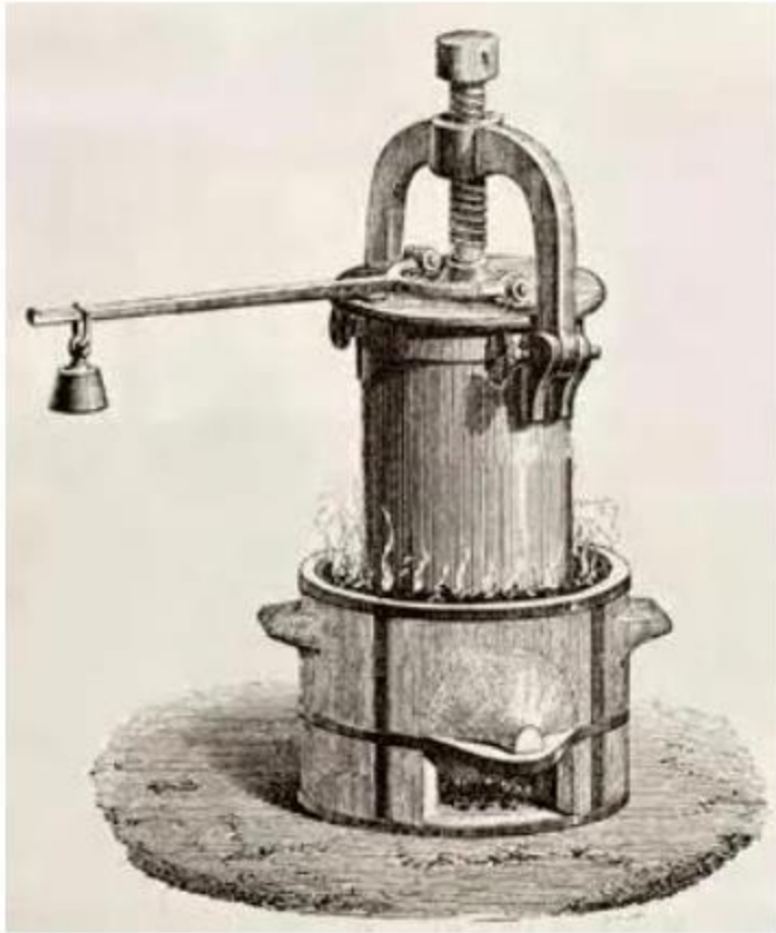
Figure 2: The first steam sterilizer built in 1880 by Charles Chamberland
