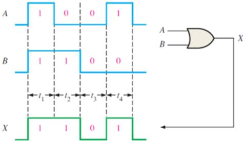
**Example:** Determine the output of the OR gate for the input waveforms shown below.
