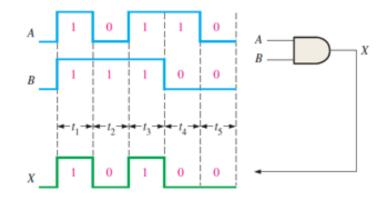
**Example:** Determine the output of the AND gate for the input waveforms shown below.
