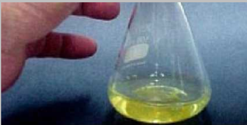
Figure 1 Before the addition of any silver nitrate the chromate indicator gives the clear solution a lemon-yellow color.
