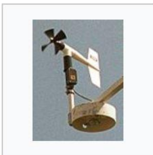
Helicoid propeller anemometer incorporating a wind vane for orientation
