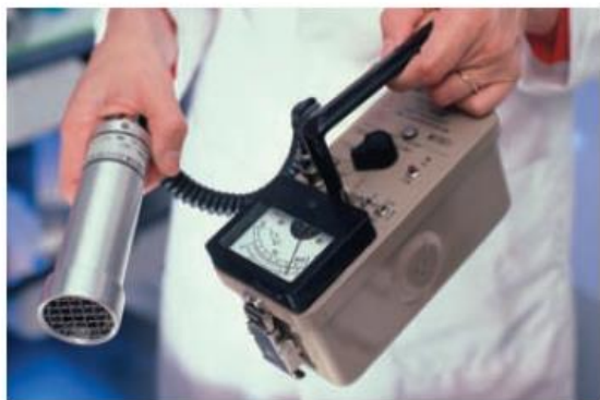
A Geiger counter is a device used to detect radiation.
