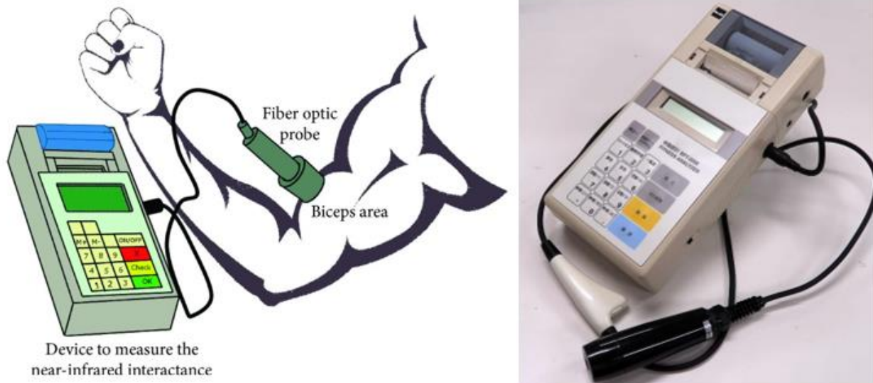
Figure (3): Near-IR spectroscopy for fat measuring.
