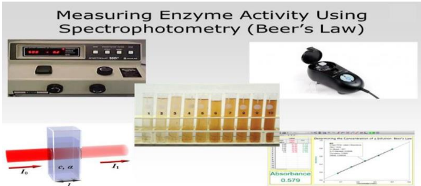
Figure (2): Measurement of enzyme using spectrophotometer.
